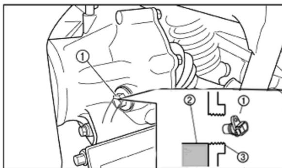
①减速箱齿轮机油加油螺栓
